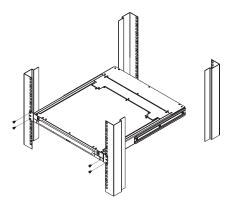
2. While the first person still holds the switch in place, the second person slides the L brackets into the switch's side mounting brackets, from the rear until the bracket flanges contact the rack, then - using the screws provided with the rack mounting kit - screws the L brackets to the rack.
